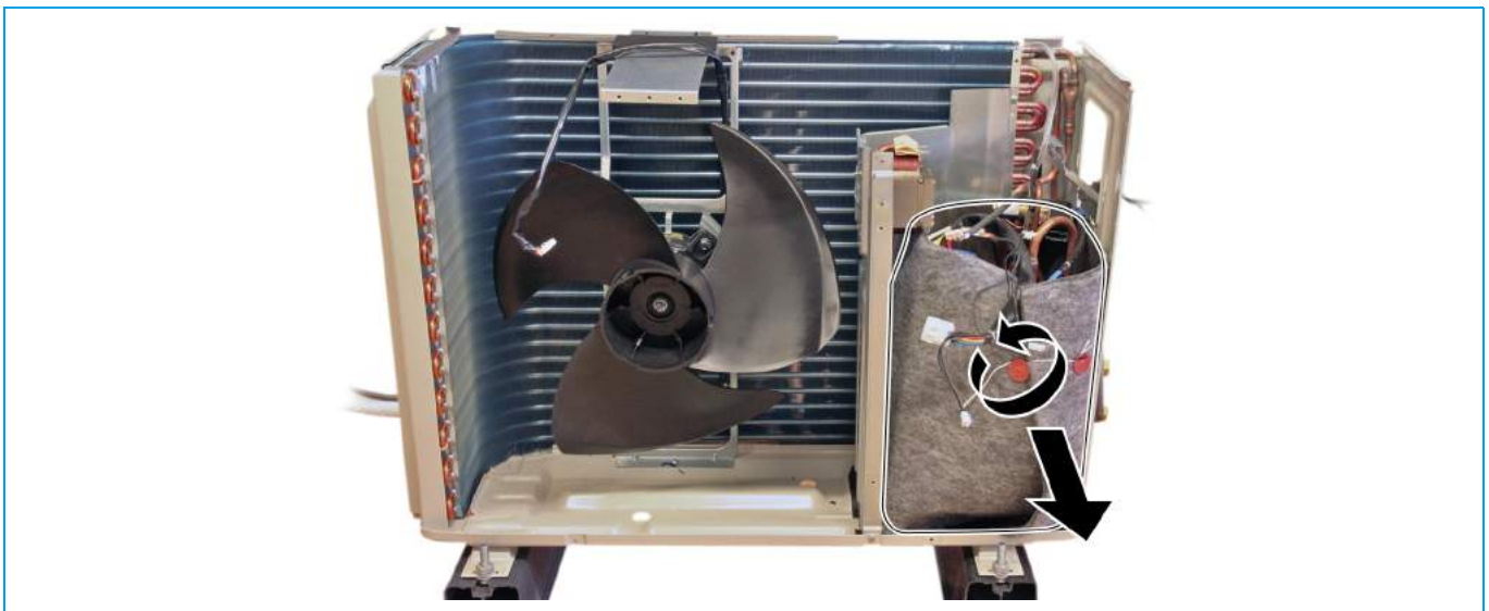
Figure 3-10: Removing the compressor sound insulation
