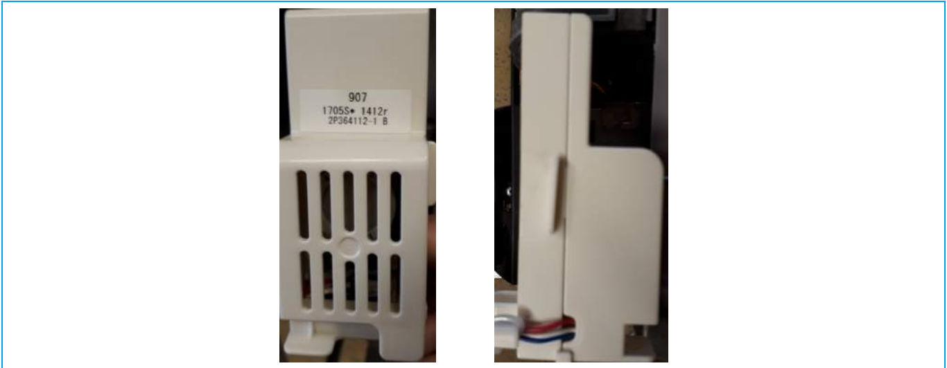
Figure 3-5: Removing casing of the sensor
